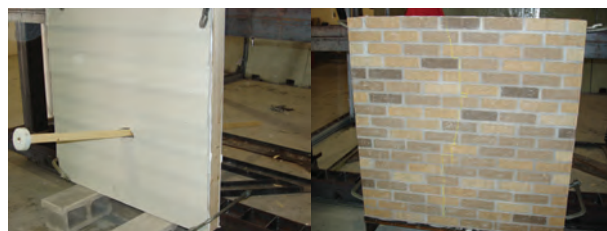
This test, conducted at Texas Tech, shows what happens during a 100-mph wind storm. The 2x4 impales the fiber cement while it merely bounces off of the brick wall.
